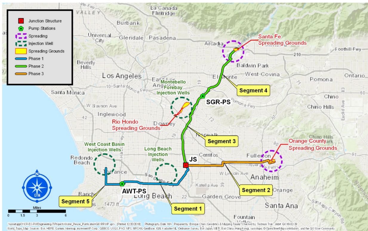
Figure 5.6: Conveyance System – Alternative E: Three-Phase Scenario (Harbor Area)
