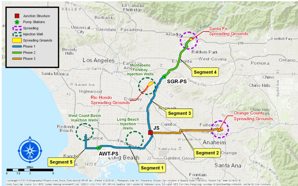
Figure 5.5: Conveyance System – Alternative D: Three-Phase Scenario (Central First)
