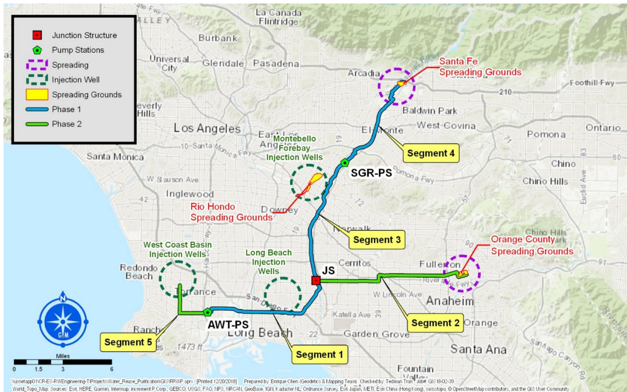
Figure 5.3: Conveyance System – Alternative B: Two-Phase Scenario (North First)
