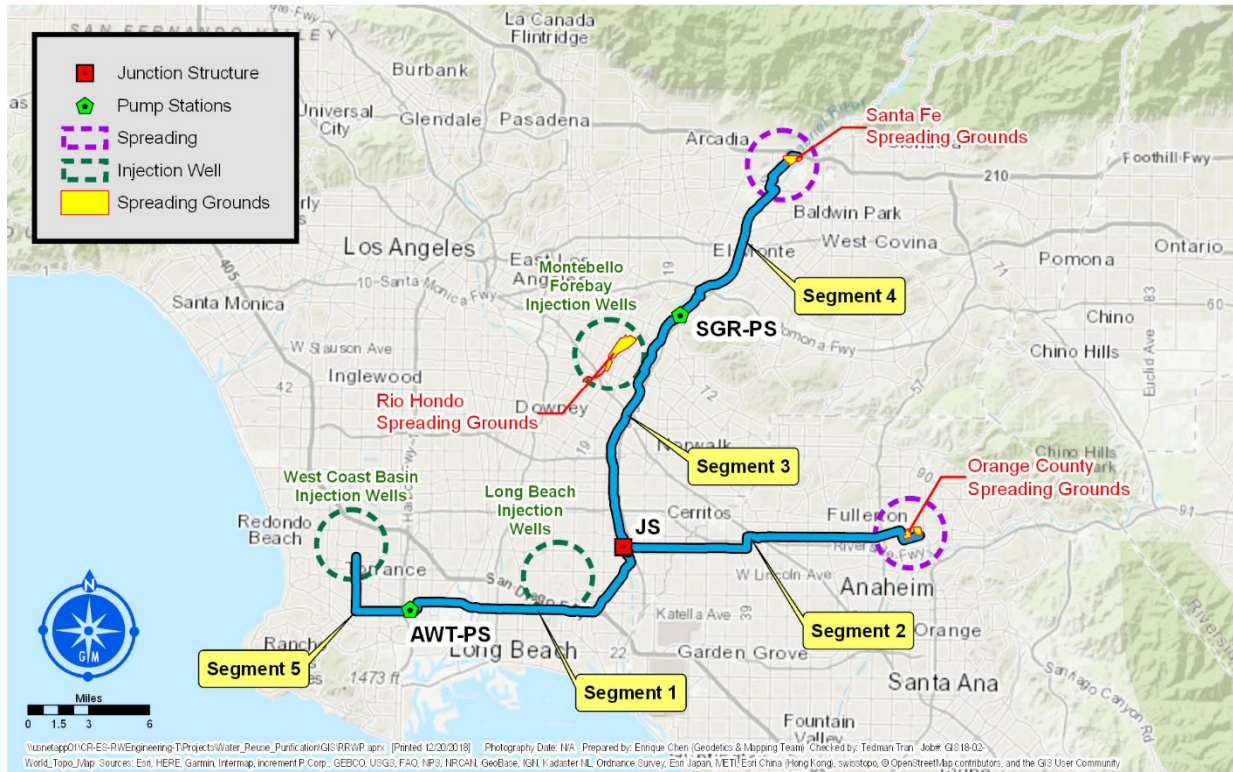
Figure 5.2: Conveyance System – Alternative A: Single-Phase Scenario (Full Program)
