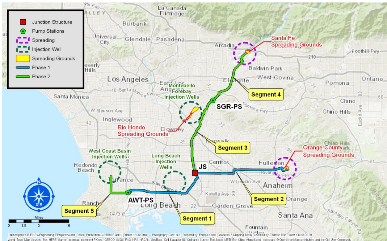
Figure 5.4: Conveyance System – Alternative C: Two-Phase Scenario (East First)
