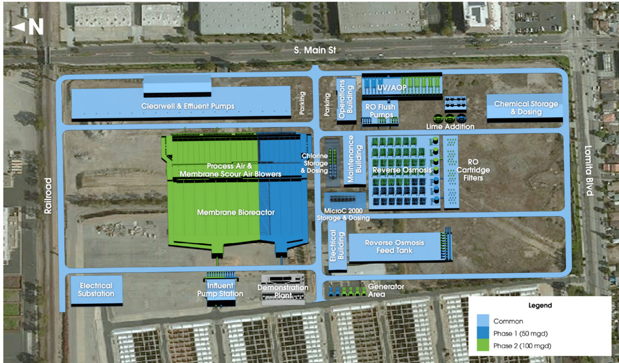
Figure 4.7: Site Plan – Alternative C: Two-Phase Scenario (East First)
