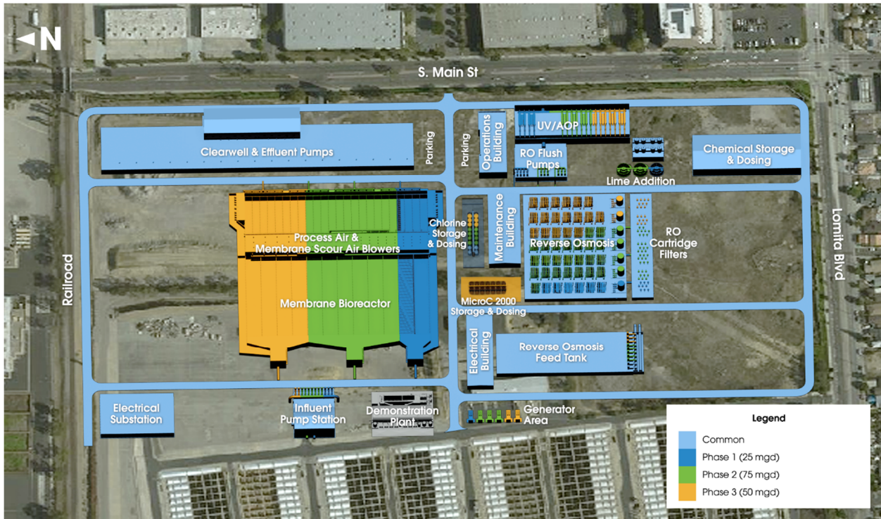
Figure 4.9: Site Plan – Alternative E: Three-Phase Scenario (Harbor Area)
