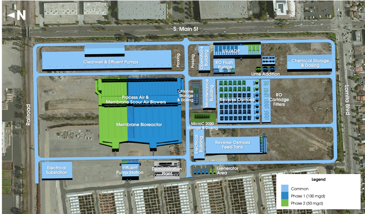
Figure 4.6: Site Plan – Alternative B: Two-Phase Scenario (North First)
