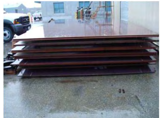
Stocks of steel plate allow Metropolitan to roll pipe of various diameters and wall thicknesses
