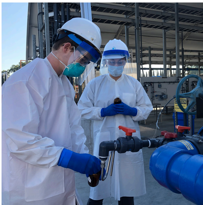
Staff collecting membrane bioreactor filtrate samples for chemical analysis at the Advanced Purification Center.
