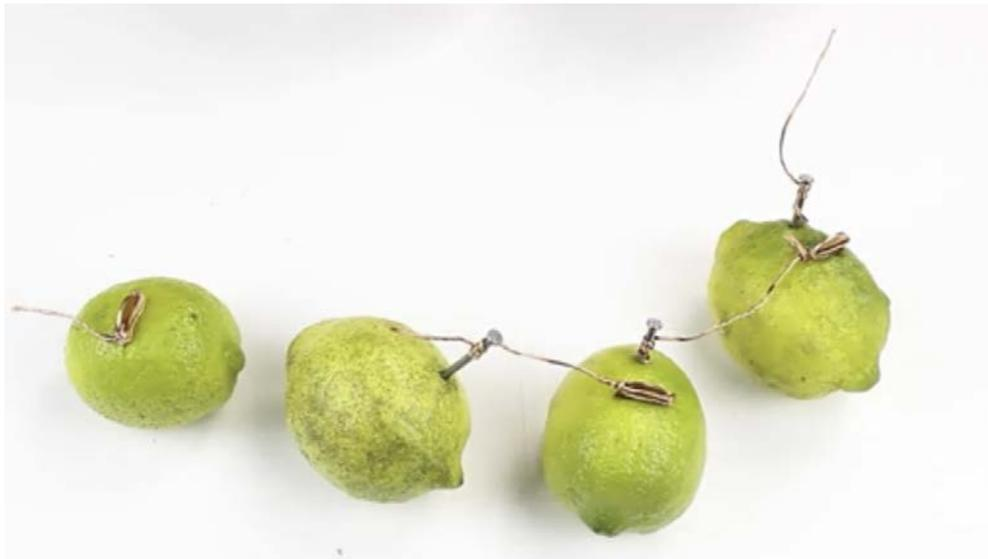
To measure the voltage, simply connect the clips of your multimeter to the free ends of the copper wires.
