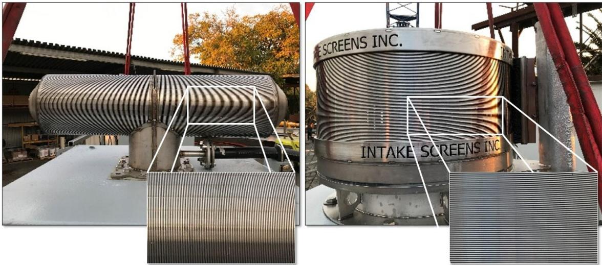
**Figure 5. Pilot-scale 1-mm passive wedgewire screen from Aqseptence (left) and pilot-scale 1-mm active wedgewire screen from Intake Screens, Inc. (right).**
