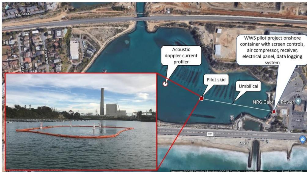
**Figure A-2. Location of the Pilot Project components. Plankton sampling was conducted at the location of the “pilot skid”. The inset photo shows the boom and warning buoys installed to mark the stand-off zone around the submerged skid.**
