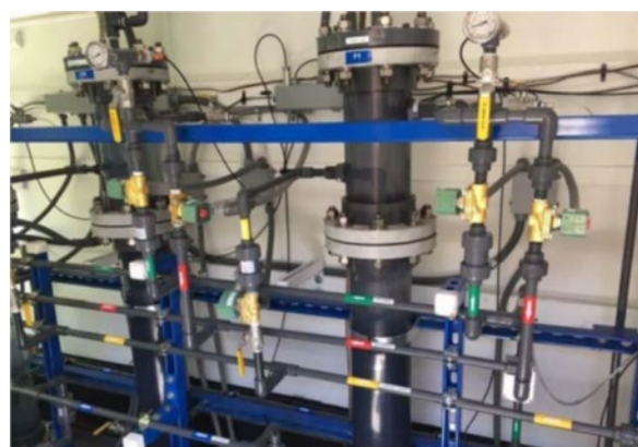
Figure 9-3. Pilot Study Filter Test Column Units setup.
